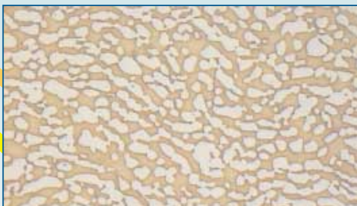
DMV 25.7 typical ferritic-austenitic microstructure, with a ferrite content of 40% to 60% (typical value is 45% to 55%).
